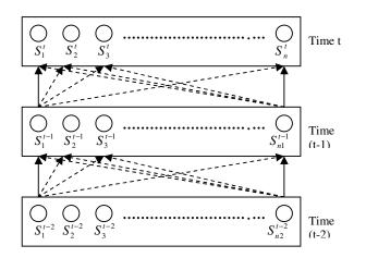
Figure 2: HMM constructed with the sensors in the last three time sequences for any particular activity. By box and arrows we indicate that all states in time (1-1) are connected with all the sensors in time l.
