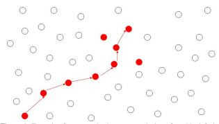
Figure 1: Example of sensor activations as user deviates from his default course of movement. Circles represent sensor and red circles represent activated sensors. Red circles connected through arrow are the default route.
