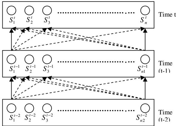
Figure 2: HMM constructed with the sensors in the last three time sequences for any particular activity. By box and arrows we indicate that all states in time (t-1) are connected with all the sensors in time t.
