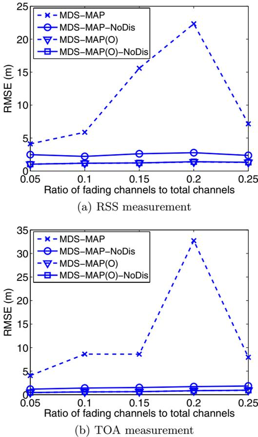
Fig. 5. Root Mean Square Error for the simulations with fading channels
