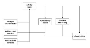
Fig. 2. Component organization: sensor data streams (left) go to visualization model to be embedded into the visual context models (center); low-level feature extraction and trend analysis combined with higher-level activity reasoning are performed by the activity engine and integrated with the context models, lastly, the visual context models are combined with activity and sensor data visualizations.
