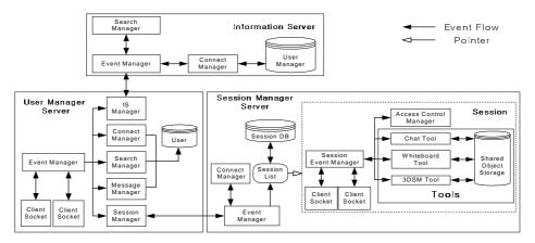
Figure 4. Collaborative System Server Architecture
