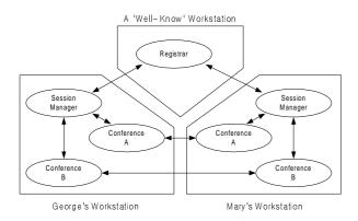
Figure 2. GroupKit's Run Time Architecture
