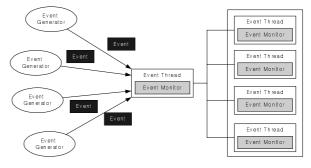
Figure 7. Extended Event Processing Model
