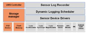
Fig. 1. Software architecture of the MASoL. There are three core components depicted on the right and components for recording life logs are described on the left.
