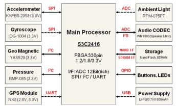
Fig. 2. System block diagram of the MASoL based on Samsung S3C2416 microprocessor. Interfaces between main processor and components are on red color. Manufactures of sensor modules are Samsung Electronics (S3C2416), Kionix (KXPB5-2353), InvenSense (IDG-1004), Yamaha (YAS529), Bosch (BMP-085), Nemerix SA(NX3) and Rohm(RPM-075PT).
