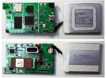
Fig. 3. Front and back side of the MASoL with battery and ZigBee communication module. The size of it is 8.5cm x 5cm and the weight is less than 50g.
