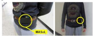
Fig. 4. MASoL has been worn by the patient. For avoiding installation error, we fixed the direction and location of the device to waist. User controls the device by three buttons(turn on/off, reset, resume etc.) above it.
