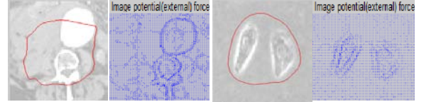
Figure 6. Sample segmentation results of active contour model (snake). If there is more than one object, and we want to segment all the objects from the image via one initial curve, so in this case the active contour snake cannot segment. The blue image shows the external force of the snake.
