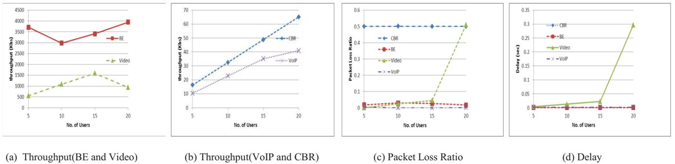
Figure 6. QoS Metrics for Vehicular Speed 120 Kmh (Single Flow: QoS Classes CBR, Video, VoIP and Best Effort)
