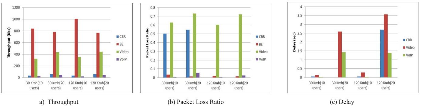
Figure 7. Comparison of QoS metrics for Vehicular Speed 30 kmh and 120 Kmh (Mixed Flows: CBR, Video, VoIP and Best Effort)
