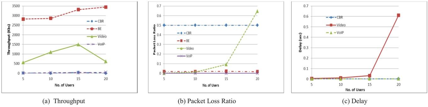
Figure 4. QoS Metrics for Vehicular Speed 3 Kmh (Single Flow: QoS Classes CBR, Video, VoIP and Best Effort)
