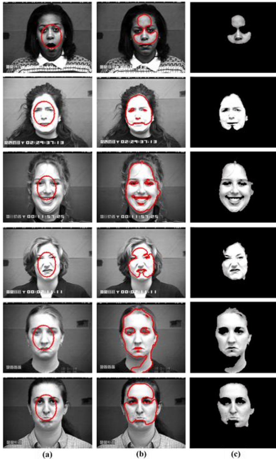
Fig. 2. Sample results of CV AC model (a) represents the initial contour (b) shows the final contour and (c) presents the extracted face.
