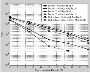
Fig. 3 Simulation MMSE algorithm in all cases with  $n_T = 4$ ,  $n_R = 4$  uncoded BPSK symbols
