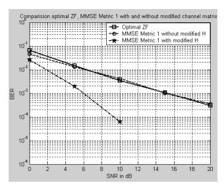
**Fig. 2** Simulation with  $n_T = 4$ ,  $n_R = 4$  uncoded BPSK symbols
