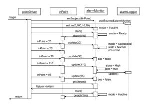
[Figure 9] Sequence Diagram of Alarm Monitoring System
