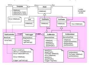
[Figure 2] Class Structure of BIT-Embedded Framework Hot Spot
