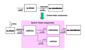
[Figure 11] Embedding BIT Components in an AlarmMonitor
