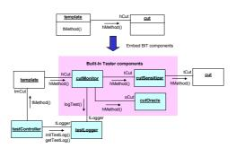
[Figure 3] Object Structure of BIT-Embedded Framework Hot Spot
