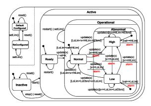
[Figure 7] State Behavior of the AlarmMonitor
