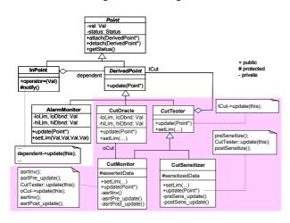
[Figure 10] Class Structure of BIT-Embedded Alarm
