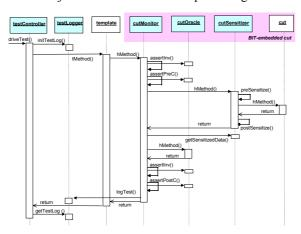
[Figure 4] Sequence Diagram of BIT-Embedded Framework Hot Spot
