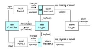
[Figure 13] Possible Object Structure of BIT-Embedded Alarm Monitoring System
