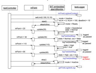
[Figure 12] Test Scenario of BIT-Embedded Alarm Monitor
