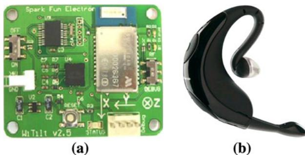
**Fig. 2** **a** Witilt v2.5 triaxial accelerometer, **b** Jabra BT250v bluetooth headset
