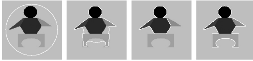
Fig. 1. CV AC failure on capturing an inhomogeneous object, \text{cpu} = 58 s. Left to right: initial ( F(C) = 645 ), intermediate (312), final (34), and desired position (197). The plot of F(C) at every iteration is given in Fig. 2.
