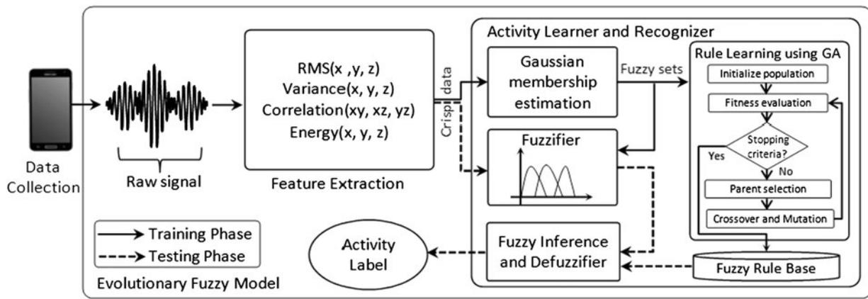
**Fig. 1** The proposed architecture of the evolutionary fuzzy model
