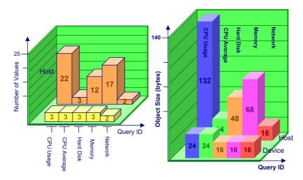
Fig. 3. (Left) Comparison between number of values at the Host and values sent to the Device; (Right) Comparison between size of intermediate results at the Host and size of results at Device.
