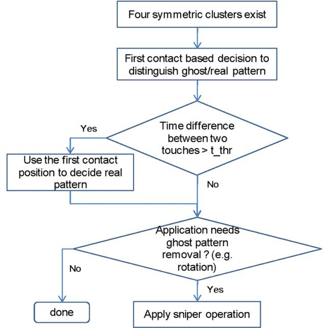
Take a 6 × 6 nP\_values presented in Table 2 as an example, which was measured with an ITO board with X and Y sensing line located at top and left side. The corresponding possible touches can be A and D or B and C similar to Figure 21. Assume that two fingers touch simultaneously; sniper should be executed as follows,
