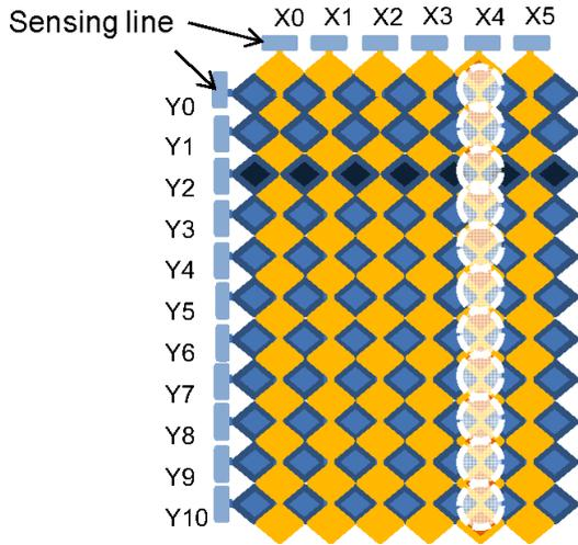
**Figure 25** Experiment result of X axis nP\_value vs. different finger positions (see online version for colours)
