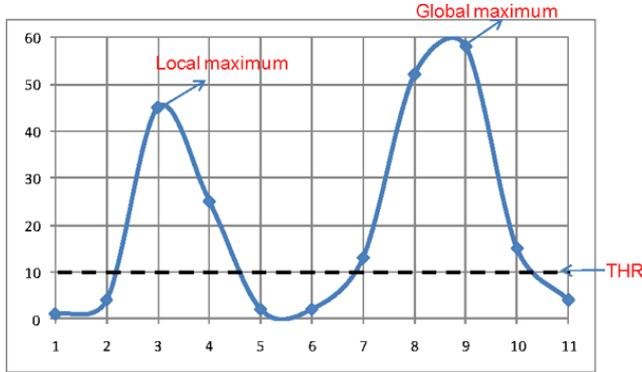
Take the above-mentioned Y nP\_value array with size = 1 as an example: [1, 4, 45, 25, 2, 2, 13, 52, 58, 15, 4], maxima-based clustering algorithm follows the steps shown here:
