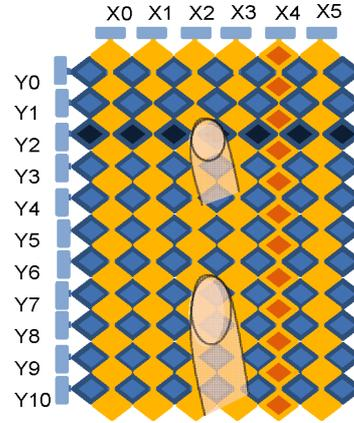
Figure 4 gives an example of nP\_value row/column data (Xi, Yj) of a 6 × 11 2-layer ITO board and marks the calculated two clusters corresponding to the actual touches on the board shown in Figure 3. The ITO board has diamond pattern with six channels in x-axis and 11 channels in y-axis. The Capacitive touch Elements (CEs), which is a notation for physical capacitive touch element), on the same X or Y channel generate the same X nP\_value or Y nP\_value.
