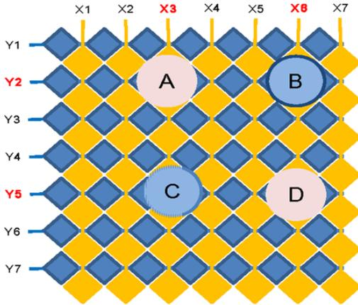
In some multi-touch applications such as rotating a picture, it can hardly distinguish the direction as clockwise or counter clockwise as shown in Figure 22 when ghost pattern exists.
