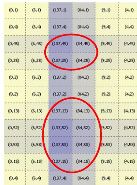
The basic idea of maxima-based clustering is to search maxima, which includes global maxima and local maxima in each x-/y-axis, respectively, and group the adjacent nP\_values, which are larger than a certain threshold together with the found maxima to form the clusters as shown in Figure 5. In case of the sample nP\_values shown
