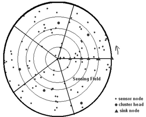
Fig. 8. Single mobile sink moving strategy in MECA
