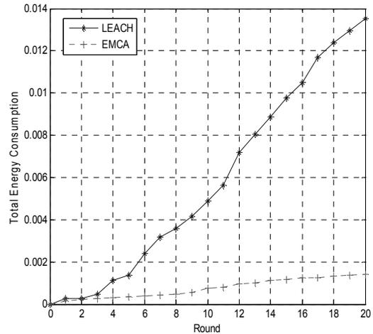
Fig. 7. Total energy consumption between EMCA and LEACH
