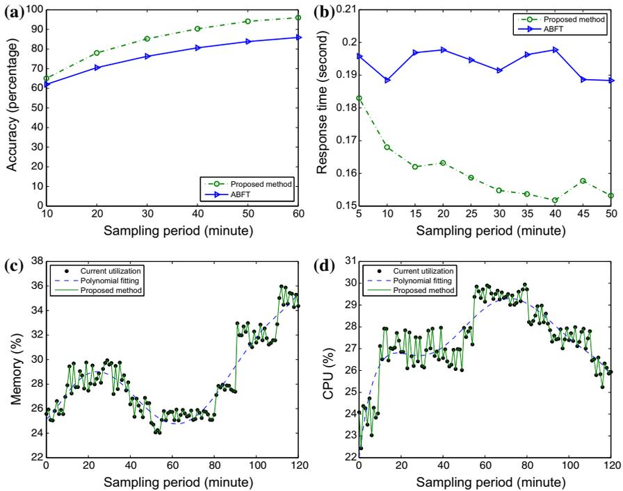
**Fig. 6** **a** Accuracy evaluation in fault detection (*higher* is better). **b** Response time evaluation in fault detection (*lower* is better). **c** Accuracy evaluation in memory utilization prediction. **d** Accuracy evaluation in CPU utilization prediction. Performance evaluation of proposed method on cloud computing system.
