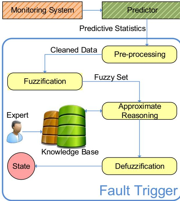
Fig. 4 Architecture of fault trigger component
