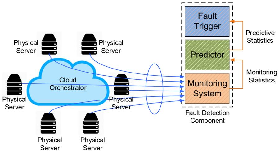
**Fig. 2** Proposed fault detection architecture
