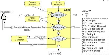
Fig. 1. Flow of Hybrid Access Control
