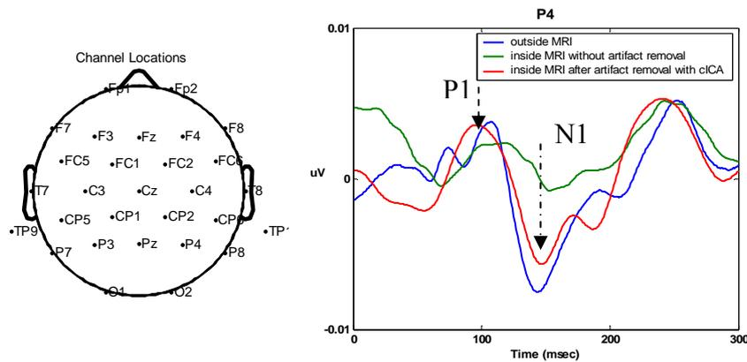
Fig. 3. Electrode locations and visual evoked potentials at P4 showing the response outside MRI (blue), inside MRI after removal (red), and with out removal (green).
