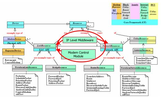
Fig. 4. UML Diagram of IP Level Middleware and Modem Control Module
