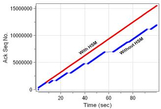
Fig. 6. Sequence number of data acknowledged by the receiver
