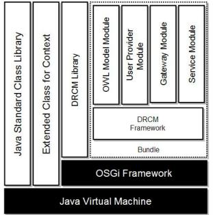
Fig. 4. Architecture of DRCM Framework
