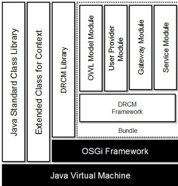
Fig. 4. Architecture of DRCM Framework
