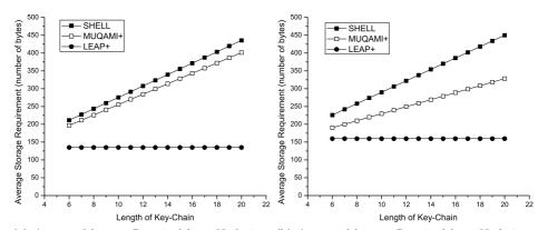
(a) Average Memory Required by a Node in a (b) Average Memory Required by a Node in a cluster of 22 nodes cluster of 38 nodes
