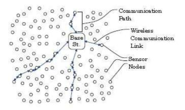
Fig. 1. Wireless Sensor Network for Soil Moisture Application. Base station is the central server in this case. Communication link between two sensor nodes can be formed if they lie within the communication range of each other.
