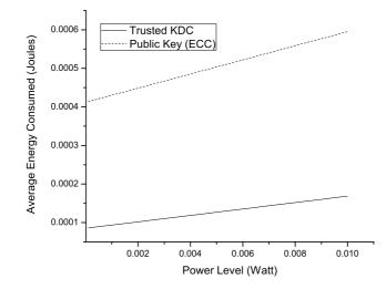
Fig. 5. Average Energy Consumed by a Sensor Node in Establishing a Key using Centralized Key Distribution Center and ECC based Public Key Cryptography while varying the Transmission Power Level (Transmission Power Level increases with the Distance between Nodes)
