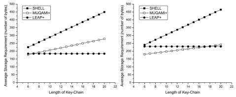
(c) Average Memory Required by a Node in a (d) Average Memory Required by a Node in a cluster of 59 nodes cluster of 110 nodes
