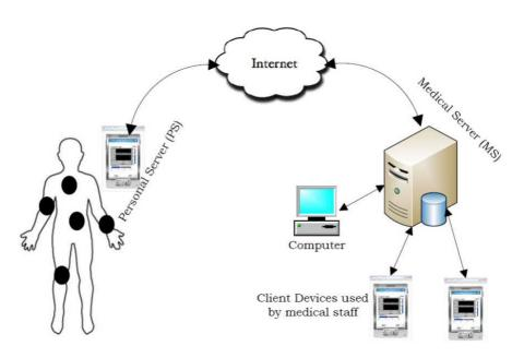
Fig. 2. Application Environment for Wireless Body Area Sensor Networks. Black circles on the body depict sensor devices used for monitoring biometrics. Sensor devices forward their readings to a PS through wireless links. PS uses wired or wireless internet connection to communicate patient's information to a MS located in a clinic or a hospital. Finally, authorized medical staff can use wired or wireless connection to access patients' real-time information on the MS.
