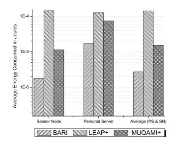
Fig. 4. Average Energy Consumed by Each Type of Node during Key Refreshment Phase of WBAN scenario
