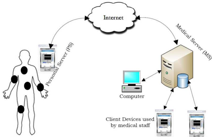
Fig. 2. Application Environment for Wireless Body Area Sensor Networks. Black circles on the body depict sensor devices used for monitoring biometrics. Sensor devices forward their readings to a PS through wireless links. PS uses wired or wireless internet connection to communicate patient's information to a MS located in a clinic or a hospital. Finally, authorized medical staff can use wired or wireless connection to access patients' real-time information on the MS.
