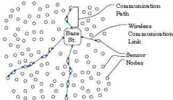
Fig. 1. Wireless Sensor Network for Soil Moisture Application. Base station is the central server in this case. Communication link between two sensor nodes can be formed if they lie within the communication range of each other.
