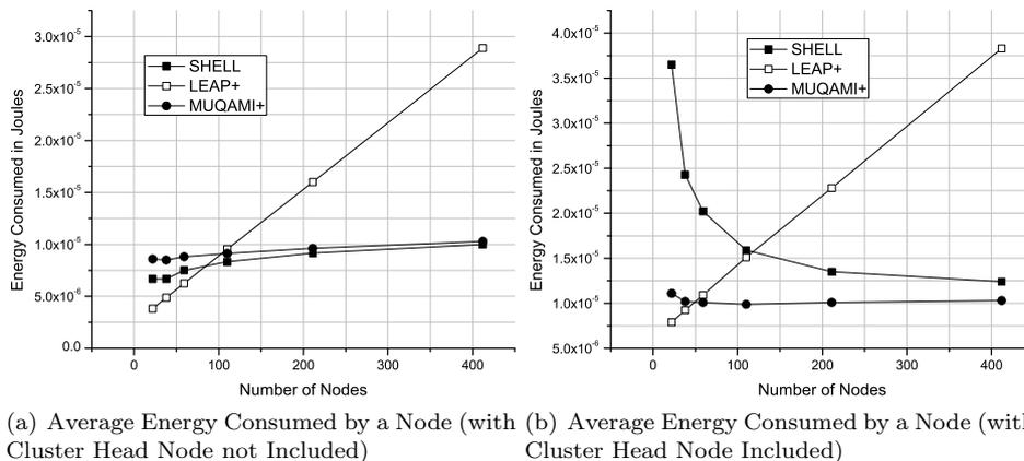
Fig. 3. Comparison of Average Energy Consumed by a Node using SHELL, LEAP+ and MUQAMI+ during Key Refreshment Phase while varying the number of nodes in a cluster
