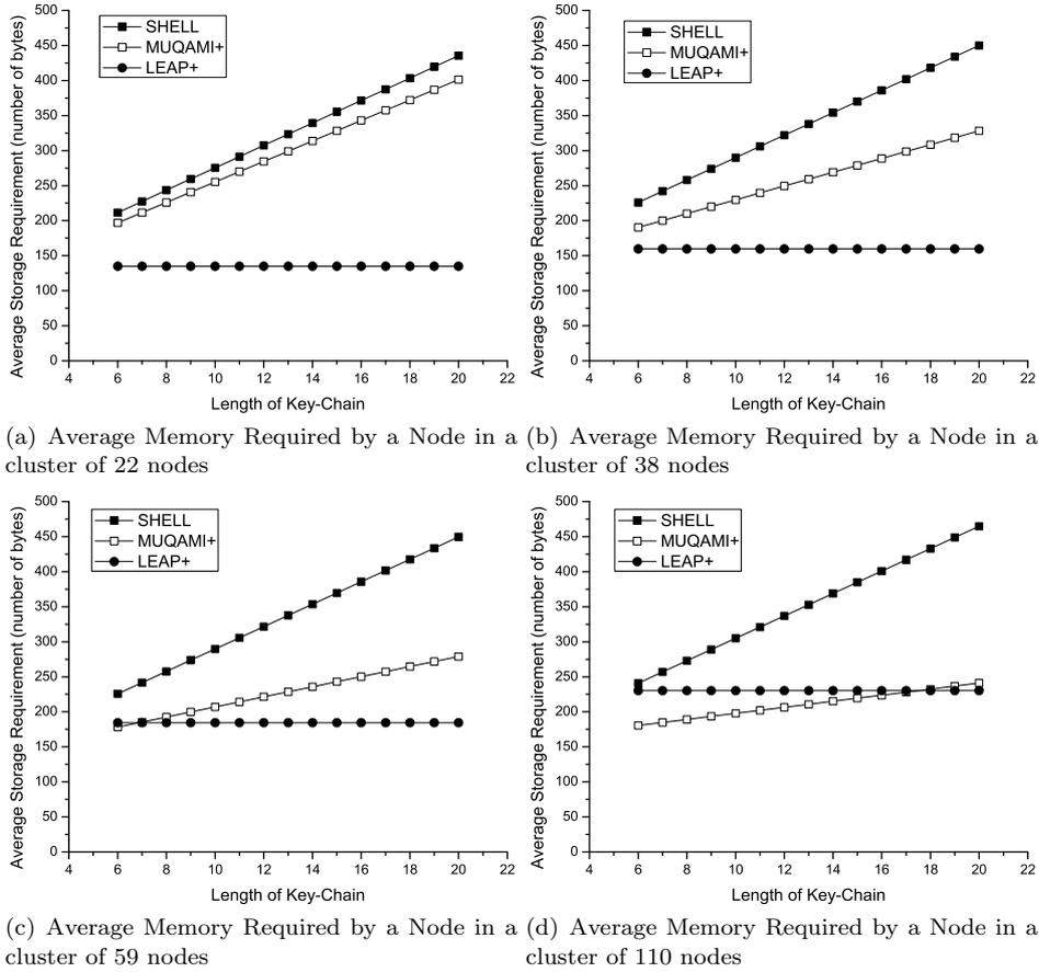
Fig. 6. Comparison of Average Storage Requirement in a Node using SHELL, LEAP+ and MUQAMI+ varying length of key-chain and node density in a cluster (High Node Density means Higher Number of Neighbouring Nodes)
