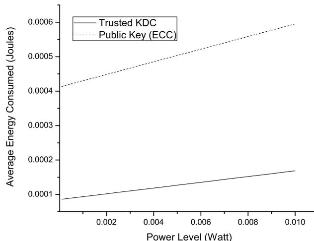
Fig. 5. Average Energy Consumed by a Sensor Node in Establishing a Key using Centralized Key Distribution Center and ECC based Public Key Cryptography while varying the Transmission Power Level (Transmission Power Level increases with the Distance between Nodes)
