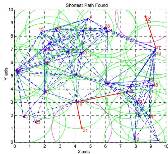
Fig. 5.10 Find shortest path by A\* algorithm from redundant node to virtual node point.
