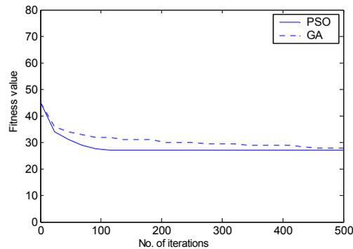
Fig. 5.5 Comparison of convergence rate between PSO and GA based on Eq. (3-12).
