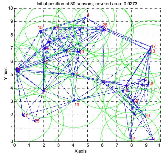
Fig. 5.8 Initial random deployment with sensing range 2m and communication range 4m.
