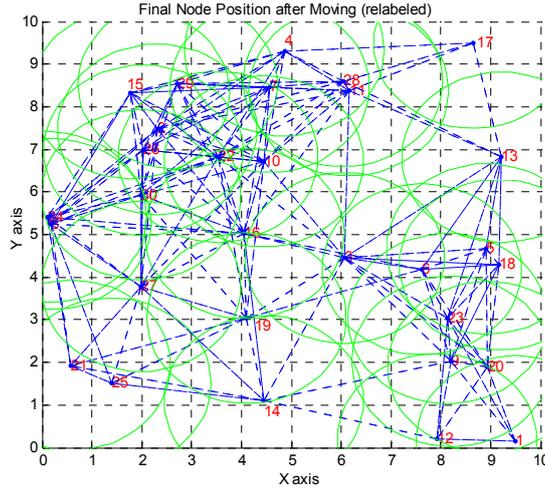
Fig. 5.11 Final node positions after executing proposed movement-assisted deployment algorithm
