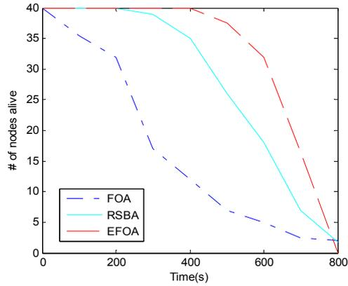
Fig. 5.17 # of nodes alive over time where each node begins with 2 J of energy. (R=4, r=2).
