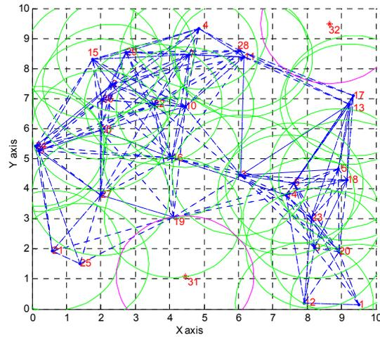
Fig. 5.9 Determine virtual node point in uncovered area and redundant nodes.
