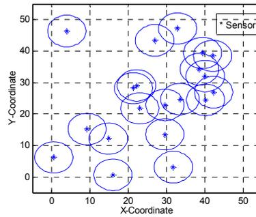
Fig. 5.3. Randomly deployed sensor network with  $r=5$  (Coverage value=0.31)
