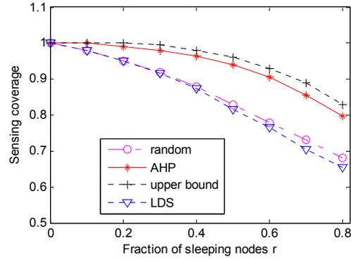
Fig. 5.30 Coverage versus the fraction of sleeping nodes.
