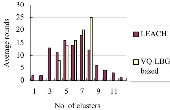
Fig. 5.27 The number of clusters in each round in both proposed algorithm and LEACH
