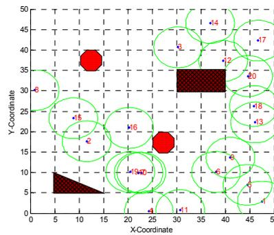
Fig. 5.19 Initial static sensor nodes placement
